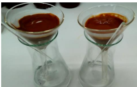
Picture 5. Separation of the iron from other metals of the mining waste extract
